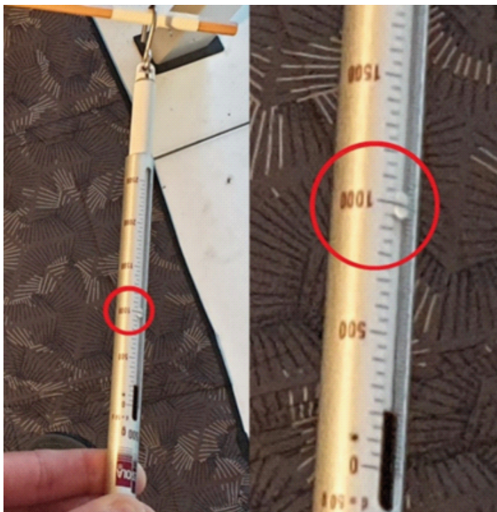
Close-up of the reading on the dynamometer
