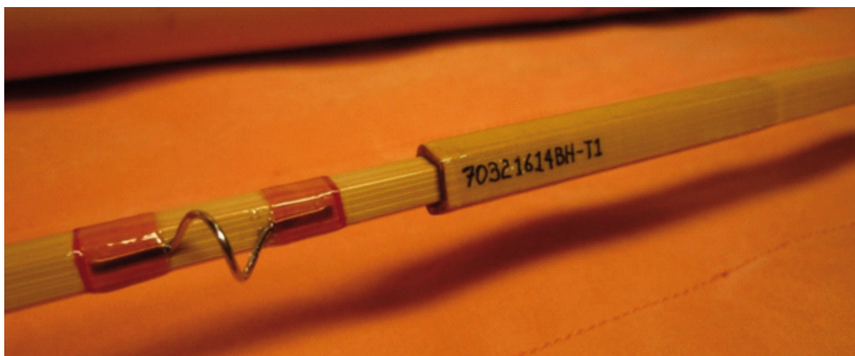
TBF hex ferrule wrapped with neutral silk
