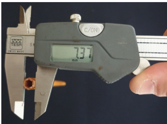
O.D. of the female measured "face to face" taken at the opening
